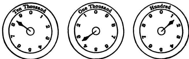
FIG. 53. DIALS OF THE GAS METER
