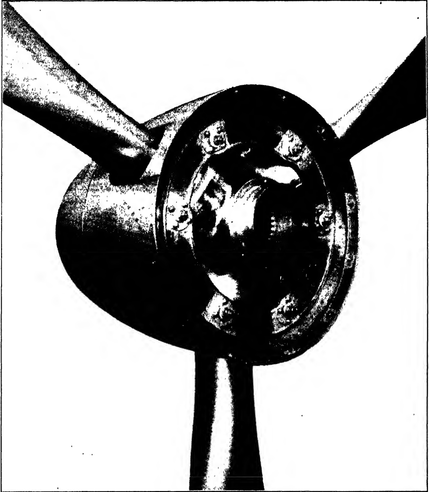
FIG. 4-15. Rear view of spinner assembly. (Courtesy Hamilton Standard Division, United Aircraft Corp.)
