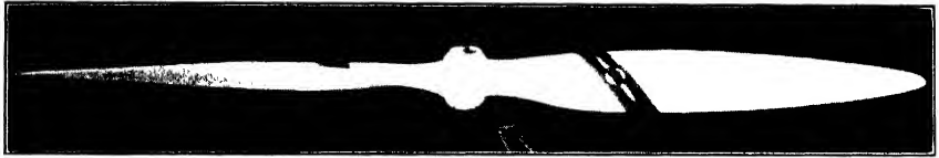
FIG. 3-3. Curtiss one-piece, aluminum-alloy propeller. (Courtesy Curtiss Propeller Division, Curtiss-Wright Corp.)
