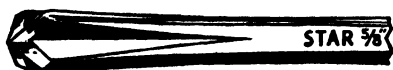
Fig. 31. Four-Point Star Drill Courtesy of Star Expansion Bolt Company, New York City
