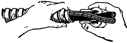
Fig. 22. Inserting Anti-Short Bushing Courtesy of National Electric Products Corporation, Pittsburgh, Pa.
