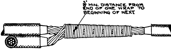
Fig. 60. Tee Tap on Small Stranded Conductor
