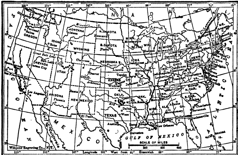
FIG. 230. — Map of asphalt and bituminous rock deposits of the United States. (After Eldridge, U. S. Geol. Survey, 22d Ann. Rept., IX.)
