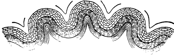
PLATE XX, FIG. 1. — Ideal section of an upright normal anticlinorium. (After Van Hise.)
