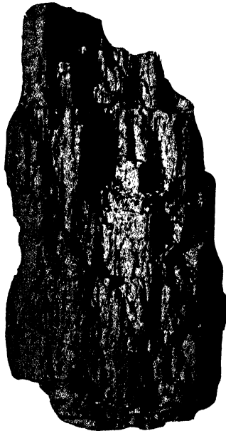
FIG. 2. — Bituminous coal, showing prismatic structure. (After Campbell, Econ. Geol., III.)
