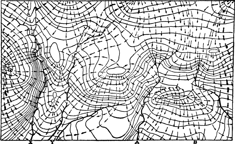
FIG. 144. — Map showing position of water table by contours (continuous lines), lines of motion of ground water (arrows), and surface streams. (After Slichter, from Fuller, Domestic Water Supplies.)
