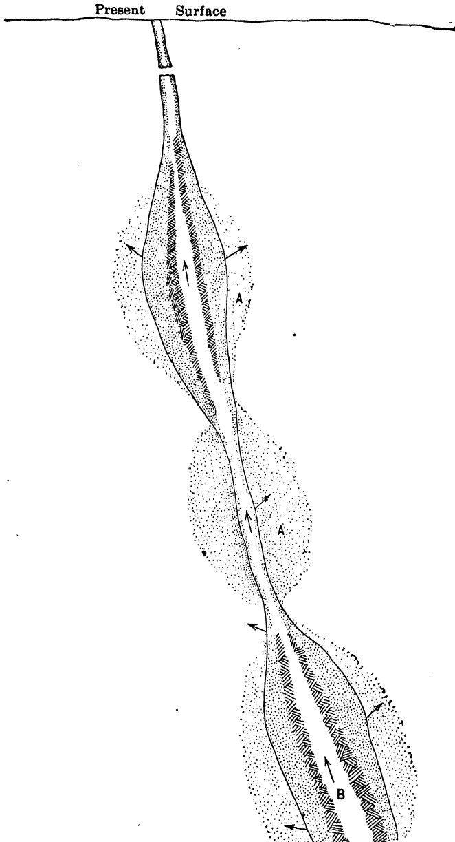
FIG. 237. — Sketch of a fissure vein indicating how deposition may take place on walls of fissure B or by replacement of wall rock A .
