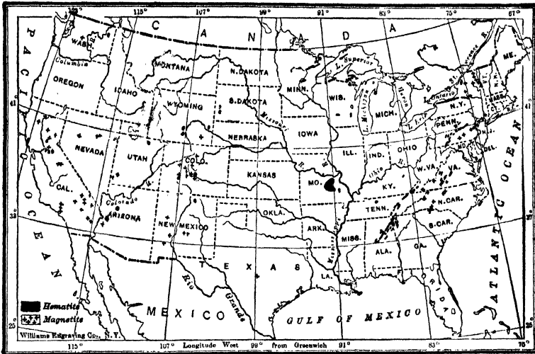
FIG. 244.—Map showing distribution of hematite and magnetite in the United States. (After Harder, U. S. Geol. Survey, Min. Res., 1907.)
