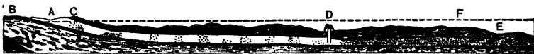
FIG. 169. — Section illustrating the transition of a porous water-bearing bed, A, into a close-textured, impervious one. Being inclosed between the impervious beds, B and C, it furnishes the conditions for an artesian fountain at D. (After Chamberlin.)
