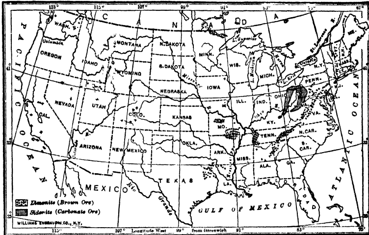
FIG. 245.— Map showing distribution of limonite and siderite in the United States. (After Harder.)
