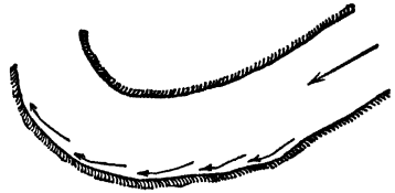
FIG. 132. — River curve indicating place of greatest erosion, on bend. (Thomas and Watt.)
