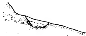
Open Ditch Intercepting Flow Normally Emerging from a Side Hill or Cut Slope
