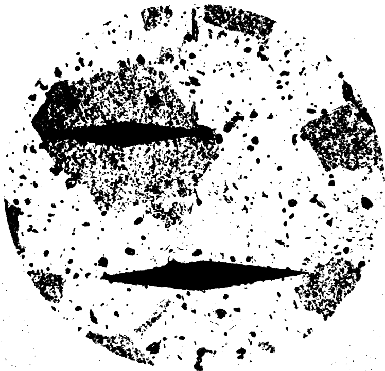
Figure 117. Knoop indentations in lead-antimony alloy, light colored material has a hardness of Knoop 6, while that of the darker colored material is Knoop 10 (250X mag.).
