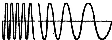
Fig. 200. —EXPONENTIAL TIME BASE PRODUCED BY INPUT DUE TO CURRENT WAVEFORMS WHEN CHARGING A CONDENSER TO ITS MAXIMUM VOLTAGE.
