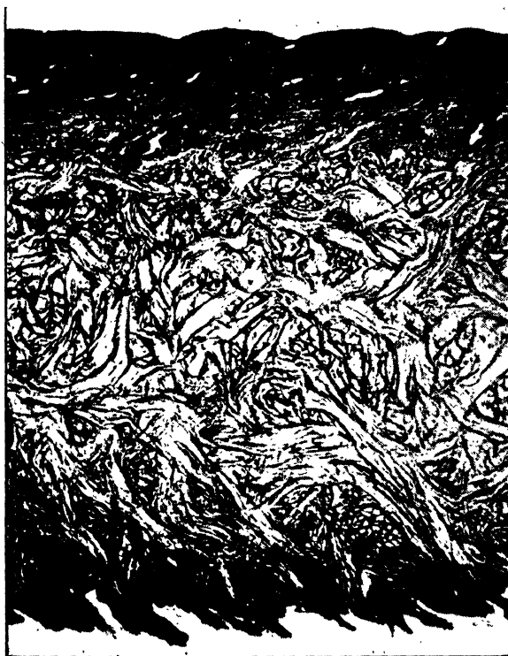
FIG. 1. Finished Calf Chrome Tanned.† Frozen section; 25\mu ; no stain; mounted in glycerin jelly; (45 \times ).
