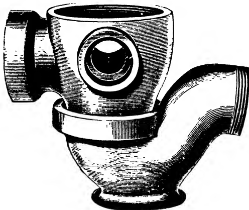
FIG. 165.—The "Kenwhar" Reversible Gully Trap.
