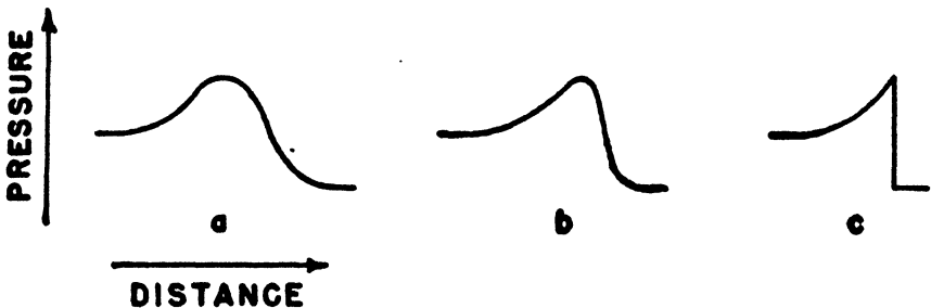
Figure 1.57. Simplified representation of development of shock wave.
