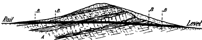
FIG. 13.—Tunnel Through an Intrusive Cill A .
