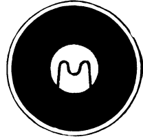
Filament too cold. Low reading.
