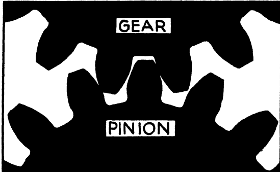
FIG. 207. CHECKING MESHING OF GEAR AND PINION
