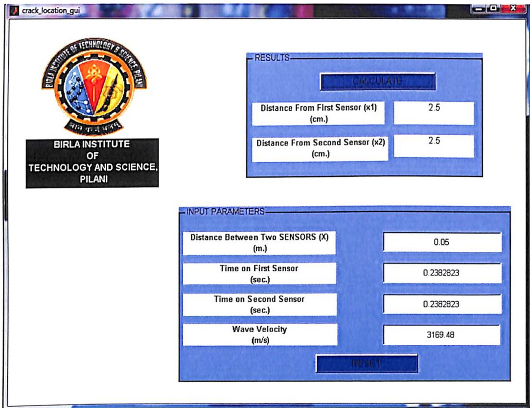
Figure 4.5 Linear location of fracture by GUI software (Distance between sensors = 5 cm)
