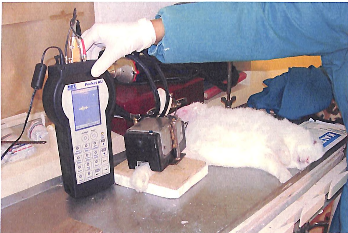
Figure 6.11 Experimental set up for Acousto-ultrasonic measurement on rabbits
