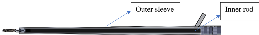
Figure 3.6: Outer sleeve enclosing the inner rod
