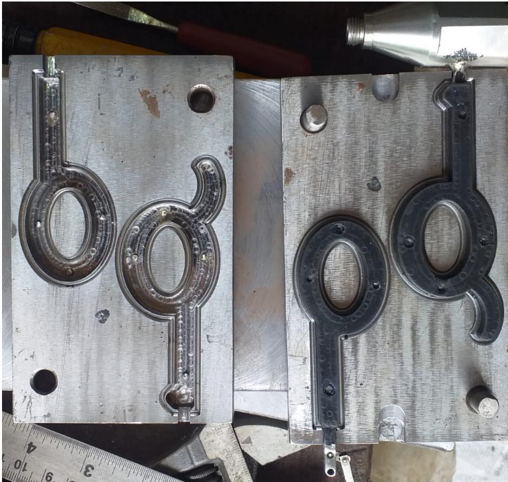
Fig. 18: Die pattern making and molding
