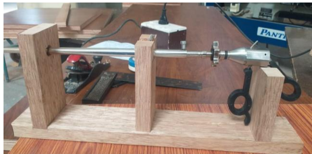
Figure 4.29: Stand for holding laparoscopic instrument in place
