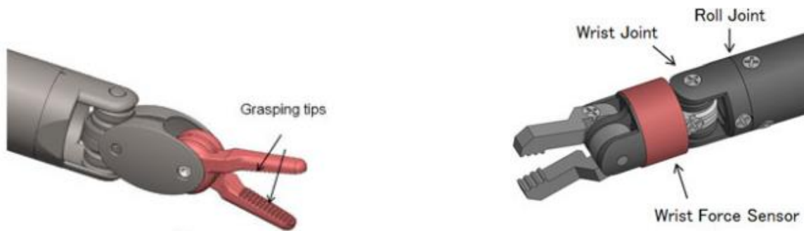
(a) Grasping Tips of the grasping instrument
