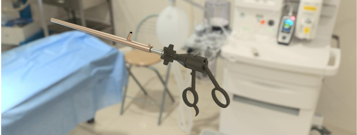
Fig. 17: SolidWorks rendering of the model of the proposed laparoscopic forceps
