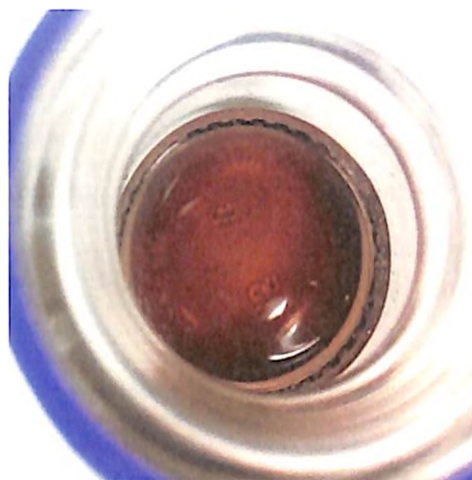
Fig. 4.15(d): Monodispersed AuNP solution using guar gum and/or \beta -CD as stabilizer
