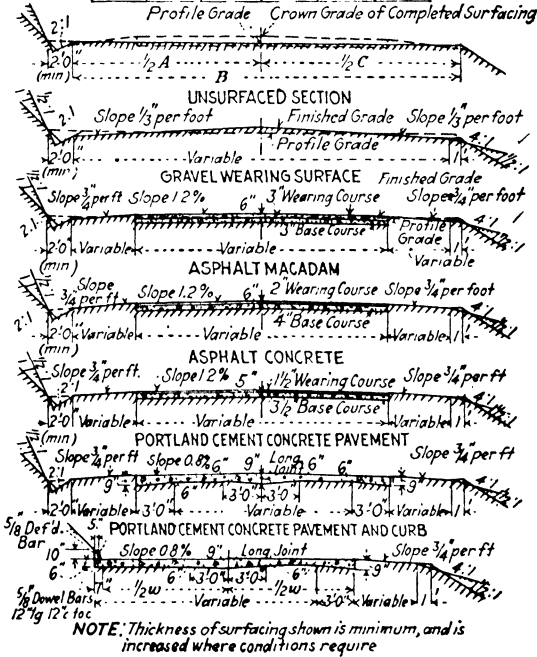
FIG. 28A.—California standard road sections (1925). (State roads.)
