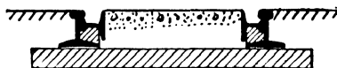
FIG. 195A.—Ordinary cold patch pavement between rails with rail grooved header. Satisfactory if surface of cold patch is kept in a smooth level plane between rails.
