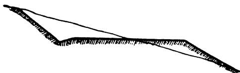
FIG. 11.—Balanced sidehill section.
