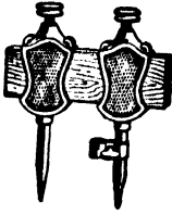
FIG. 132.—Trammel points. ( Courtesy of Stanley Tools. )
