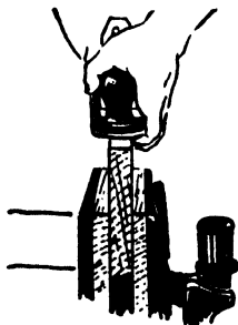
FIG. 129—Method of using smoothing or jack plane. (Courtesy of Stanley Tools.)
