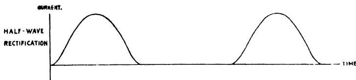
FIG. 237.—Output from half-wave rectifier.
