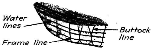
FIG. 124A.—The intact model, showing water lines, buttock lines, and frame lines painted on the outside where they intersect the shell.
