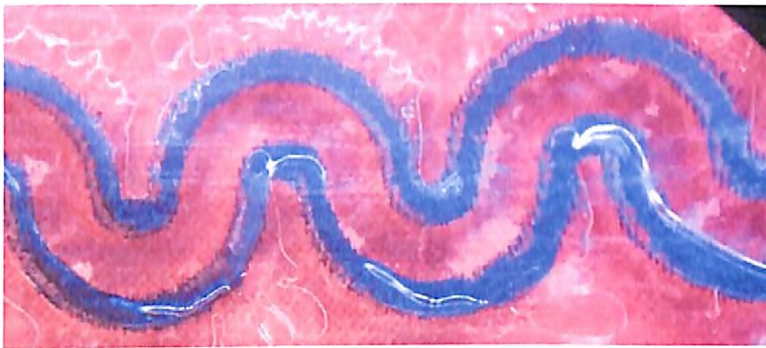
(a) Trapped dead cells at 300 kHz
