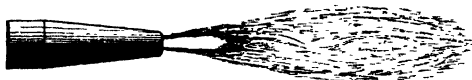
FIG. 23.—More Oxygen Pressure Applied. Flame Contains Slight Excess of Acetylene, and is Known as “Carbonizing.”
