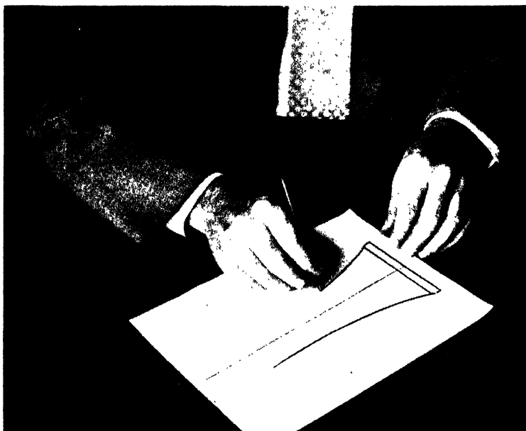
Fig. 41. Drawing a Curved Line or Arc of Large Radius by Swinging the Pencil from the Elbow which Serves as a Pivot
