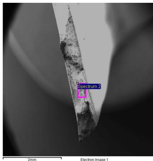
Figure 3.19 Fractography sample location of deformed test specimen
