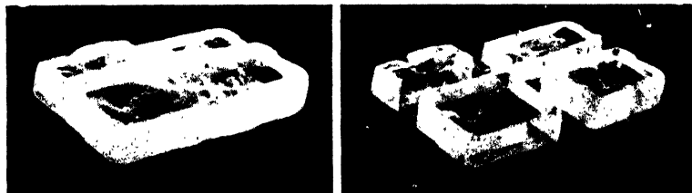
X1B. Fragment of Iceland spar (crystallised calcium carbonate) which has been cleaved by a tap from a blunt knife into four pieces, each with the same angles as the original fragment.
