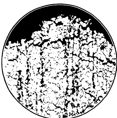
FIG. 95(b).—Creep Specimen. 9000 lb. per sq. in., 4788 hr. for rupture. Note intercrystalline fracture, and lack of strain-hardening.
