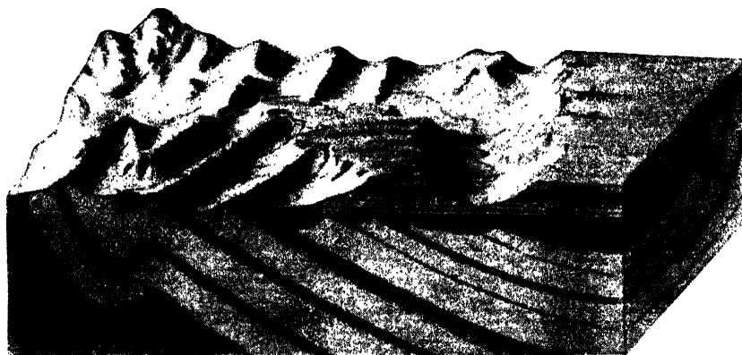
20. Geologic dating of crustal deformation. The diagram, which represents part of the eastern border of the Rocky Mountains, shows two sequences of stratified rocks having discordant structure. The tilted and folded beds were truncated by erosion before deposition of the horizontal overlying series. Hard rocks of the folded series make hogbacks, and weak strata form monoclinial valleys. The deformed and eroded rocks were buried beneath younger deposits and then subsequently exhumed partly. The geologic date of the folding must be later than the youngest deformed stratum and older than the lowermost horizontal deposit.
