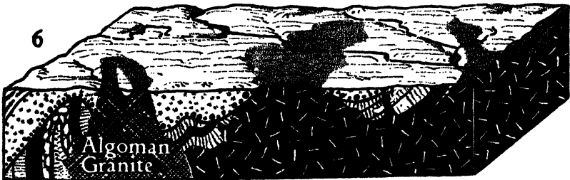
55. Pre-Cambrian geologic history of the Canadian Shield region (continued). (4) Deposition of the Timiskaming sediments on the peneplain began when sinking of parts of the land led to submergence by the sea and uplift of adjacent country furnished sediments, which include pebbles worn from the Keewatin lavas and Laurentian granite. (5) Mountain building at the close of Timiskamian time profoundly disturbed both the Timiskaming and underlying older rocks, and intrusion of granite, called "Algonian," intersected them. (6) Peneplanation that truncated the rock structure is recorded by another major unconformity.
