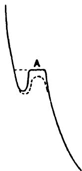
FIG. 103.—Effect of undercooling on cooling curve.
