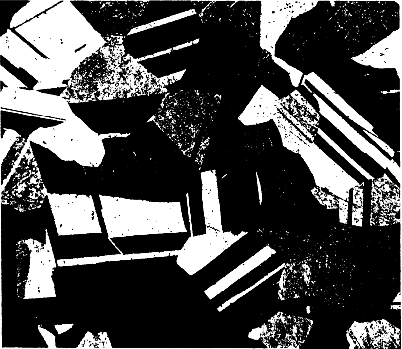
B. a- Tin-copper alloy, annealed. \times 165
