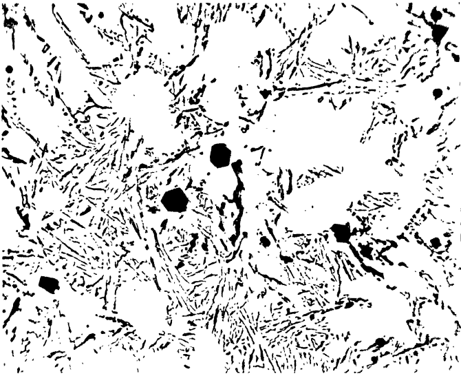
A. Aluminium-silicon alloy. Unmodified. \times 350
