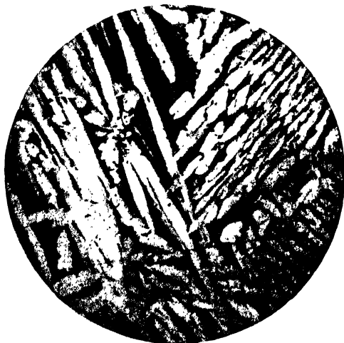
B. \alpha - \beta Aluminium-copper alloy. × 200
