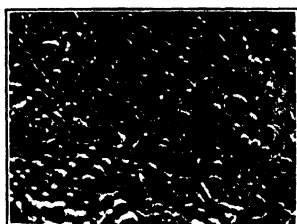
FIG. 1.—Surface of cast copper, 30 diameters.
