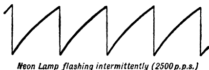
Neon Lamp flashing intermittently (2500 p.p.s.)
