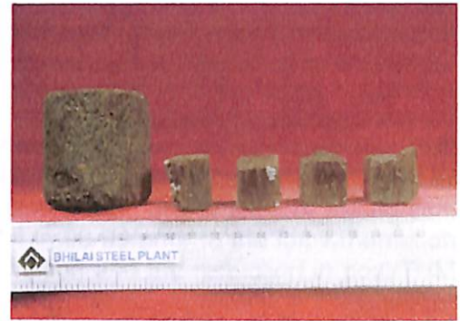
Figure 5.1: Photo and Microstructure* of Coke Breeze Agglomerate (*Magnification: 200 times, Optical Microscope - Jenapol, Camera –Contax 167MT)
