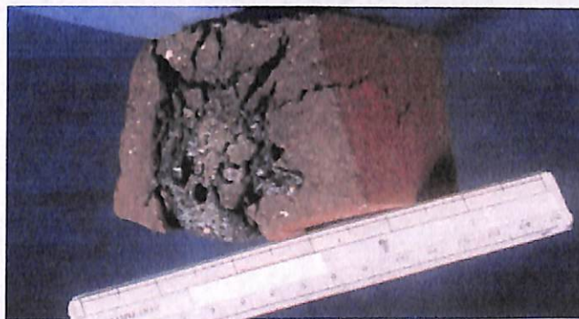
Figure 6.10: Mixed Pond-Ash Clay Bricks after Curing at 1200°C
