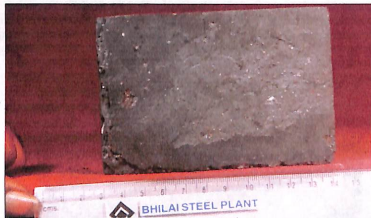
Figure 6.8: Normal Fly Ash Brick Manufactured Using FA, Clay and Lime Binder
