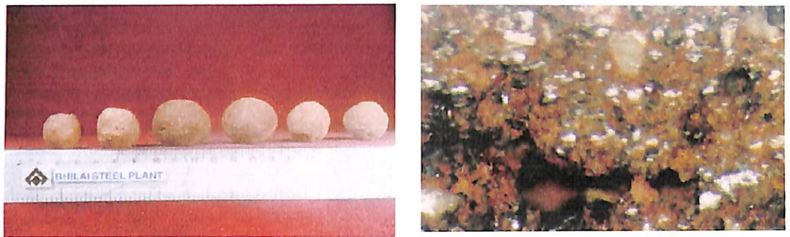
Figure-6.1: Photograph of Pellets and Microstructure* of Samples of ESP Micro Fines (*Magnification: 200 times, Optical Microscope - Jenapol, Camera –Contax 167MT)
