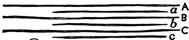
(357) END REINFORCEMENT OF BOWSTRING STRANDS
