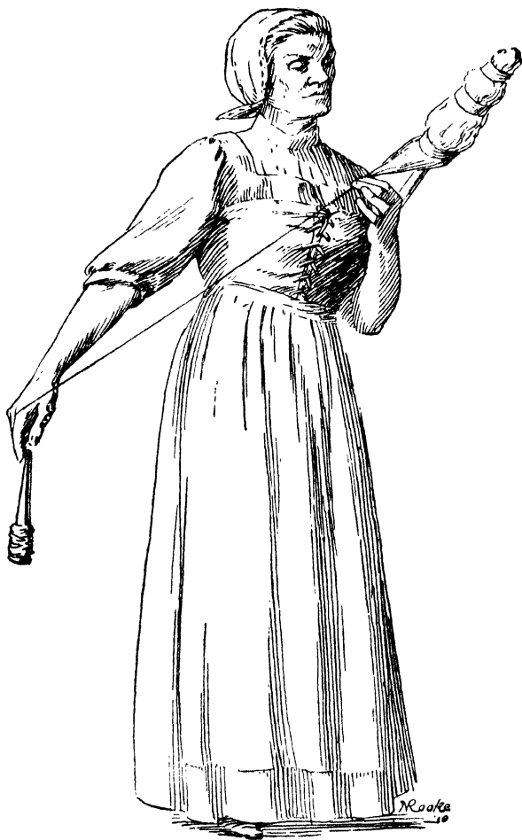
FIG. 5.—Spinning with Distaff and Spindle.
