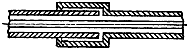
FIG. 27-22.—A short-circuited line in series with the outer conductor of a coaxial line.
