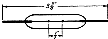
FIG. 24-8.—Gas-filled load lamp for ultrahigh frequencies.
