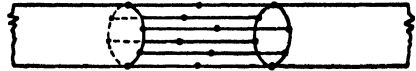
FIG. 24-5.—Arrangement of parallel thermocouples to prevent impedance discontinuity in the coaxial line.
