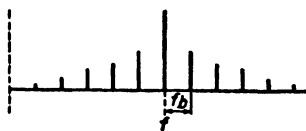
FIG. 230 Representation of disturbing output frequencies resulting from tube curvature effects in single side-band reception. Carrier frequency f_c is broken line at the left. The spurious l.f. disturbing frequency is f_b , while the desired output l.f. is |f_c - f| . The resulting interfering spurious output frequencies are |f_c - f \pm f_b q| , q being an integral number, and are shown in the diagram with decreasing amplitudes for higher values of q .
