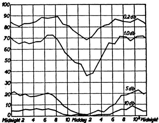
FIG. 23c Daily variations of amplitude of field-strength variations. Vertical scale: Percentage of time during which the hourly variation of field-strength amplitude is above the values indicated at the curves. Horizontal scale: Time. Conditions as in Fig. 23b. Same authors.
