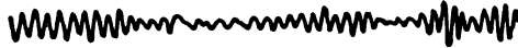
FIG. 35 Representation of spontaneous fluctuations corresponding to a frequency interval \Delta f approximately equal to \frac{1}{4} of its average frequency, round which it is centered.
