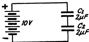
FIG. 32.—When capacitors are connected in series the total capacitance is less than that of any of them: \frac{1}{C} = \frac{1}{C_1} + \frac{1}{C_2} + \frac{1}{C_3}
