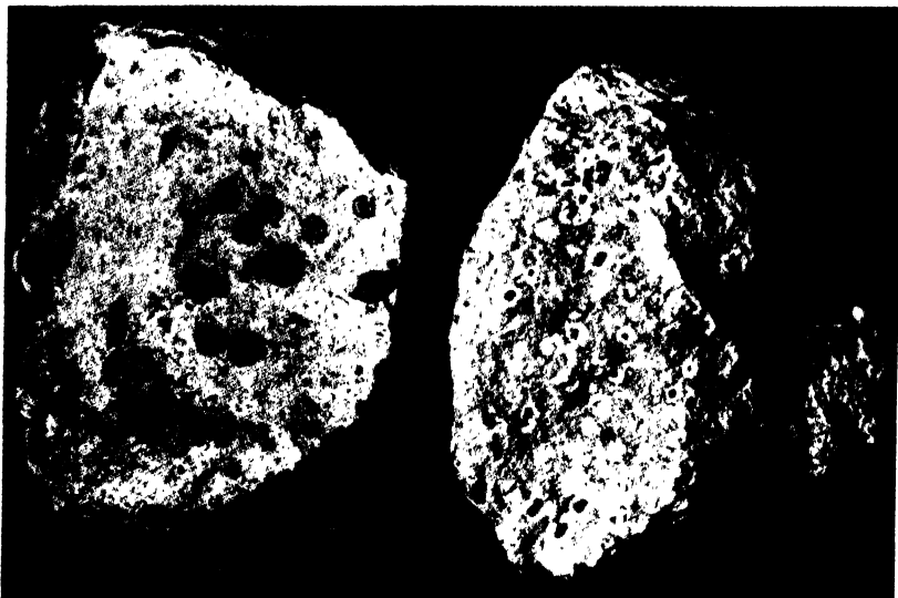
Fig. 59—Oxidation of pyrite in monzonite. Left: In slightly kaolinized monzonite. Incompletely kaolinized feldspars tend to neutralize acid and precipitate a strong limonite halo. Niagara Gulch, Bagdad, Arizona. Right: In well-kaolinized monzonite. Less effective neutralizer permits migration of iron outward through inner bleached zone. Alum Creek, Bagdad, Arizona. (After Blanchard and Boswell, Economic Geology )
