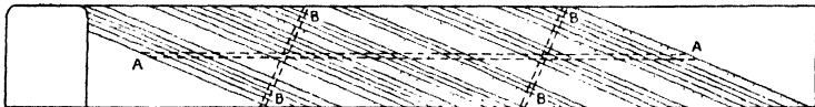
Fig. 7—Channels for sampling gently dipping formation in a crosscut. (Vertical section) Either the inclined channels, B-B, or the horizontal channel, A-A, would be proper. B-B requires less cutting; A-A may be more convenient.
