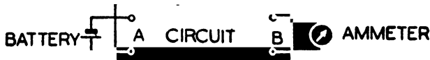
FIG. 92. THE CURRENT IS THE SAME IF BATTERY AND AMMETER ARE INTERCHANGED WHATEVER THE CIRCUIT
