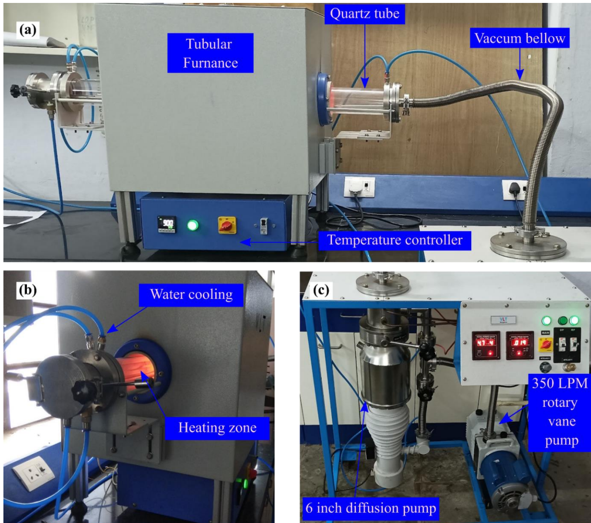
Fig. 6.3 Experimental facility a) front view, b) side view of the high-temperature vacuum furnace, and c) vacuum system
