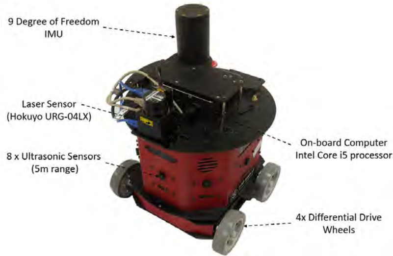
Figure 4.12: Firebird-VI Robot Equipped with HOKUYO URG-04LX-UG01 2D Laser Scanner for Real Robot Experiments
