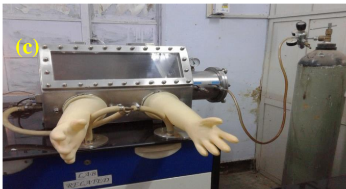
Fig. 2.1 (a) A picture of the composite pellet with electrodes, (b) A picture of Swagelok cell used for battery testing, and (c) Glove box (MTI) filled with Argon for fabrication.
