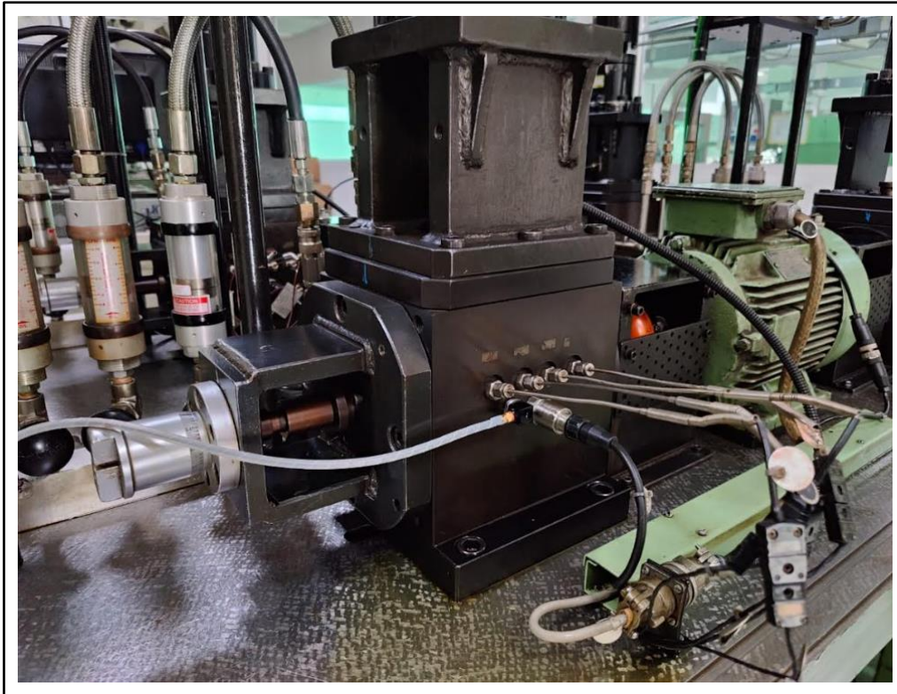
Figure 5.4 Sensor Mounting and Bearing Housing.
