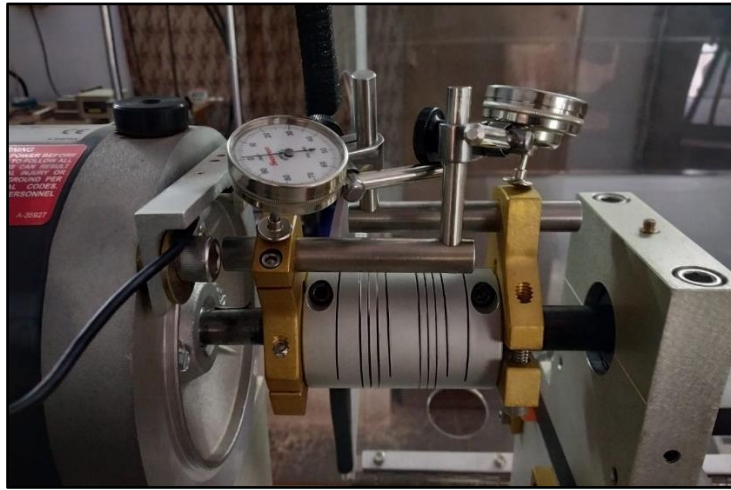
Figure 4.17. Reverse Dial Indicator
