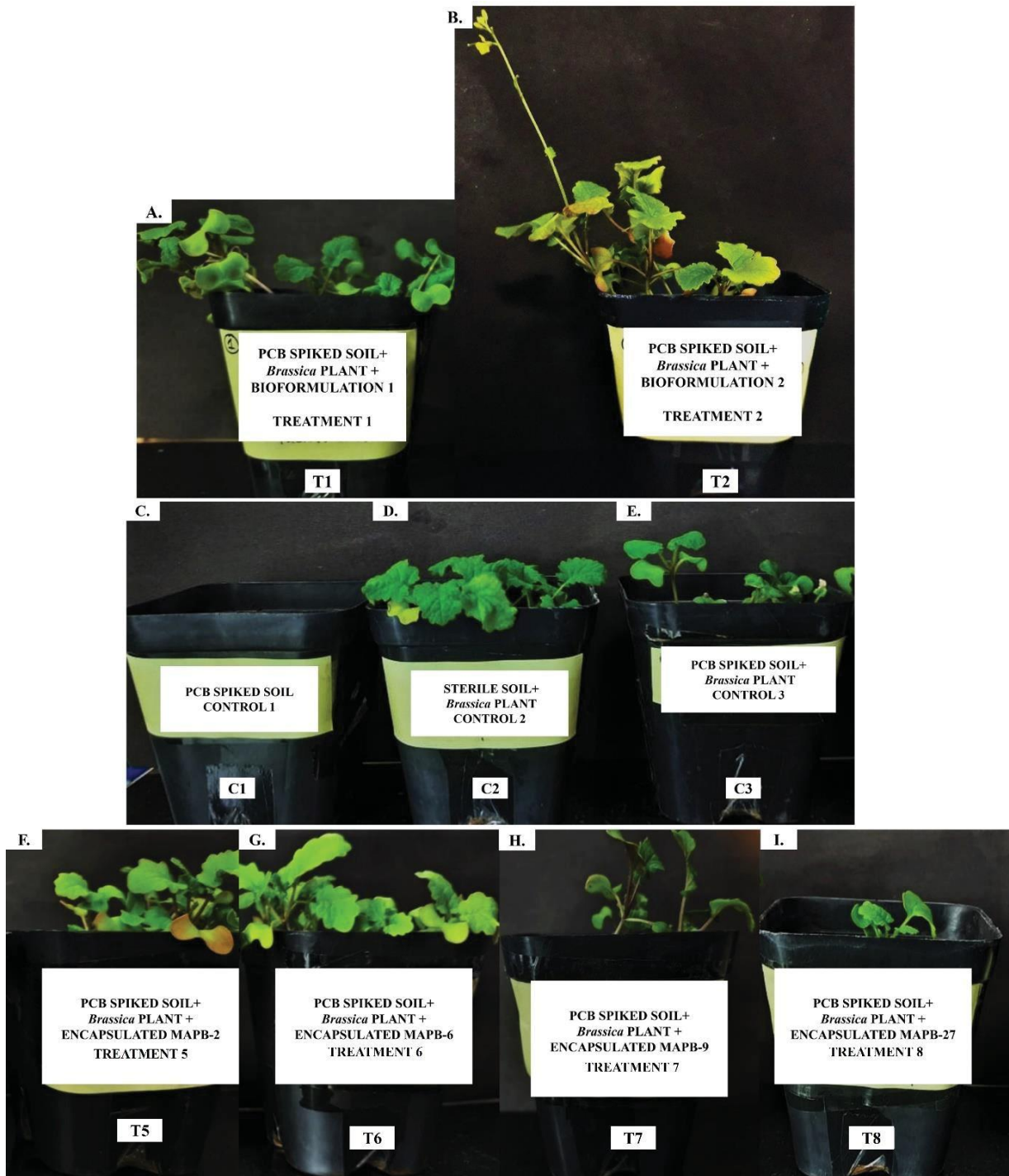
Fig. 5.6. Pot study of B. nigra growth in various bioformulation treatment and control groups. (A) T1: bioformulation with consortium #11 in ratio 1:1:1:1; (B) T2: bioformulation with consortium #11 in ratio 1:1:2:2; (C) C1 Control with PCB congener spiked soil; (D) C2 control having sterile soil with the plant (E) C3 control with PCB congener spiked soil and plant (F) T5 encapsulated MAPB-2 with spiked soil and plant; (G) T6 encapsulated MAPB-6 with spiked soil and plant; (H) T7 encapsulated MAPB-9 with spiked soil and plant (I) T8 encapsulated MAPB-27 with spiked soil and plant. The pot study was conducted for 45 days.
