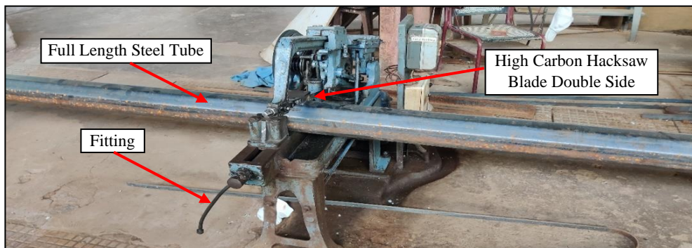
Fig. 3.8 Cutting of steel tubes as design length
