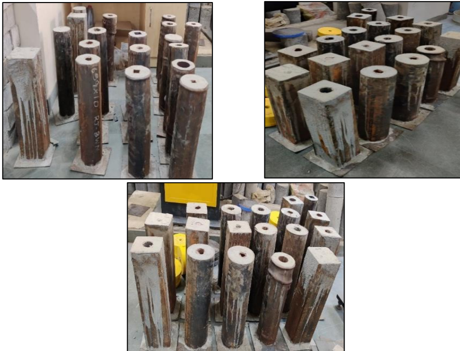
Fig. 3.14 CF DST Specimen after Placing of Concrete
