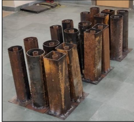
Fig. 3.13 CF DST specimen before placing of concrete
