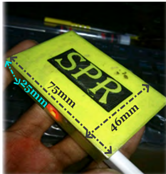
FIGURE 6.9: A miniaturized handheld version of the SPR device.
