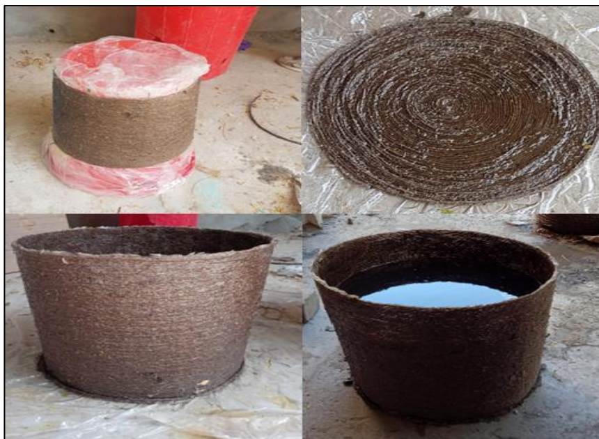
Figure 3-4 Dia of twine rope (sutli) – 2mm and the size of the model – 1.5ft dia & 2ft height
