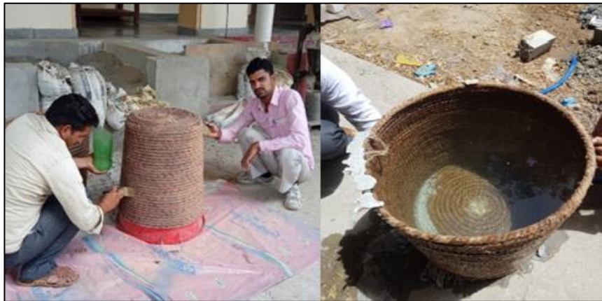
Figure 3-2 Dia of jute rope – 20mm and the size of the model – 1.5ft dia & 2ft height
