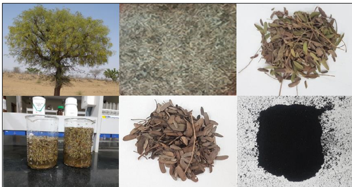
Figure 4-1 Step by step process of adsorbent preparation
