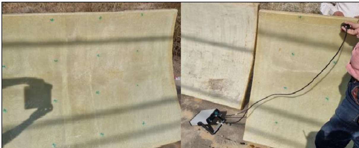
Figure 3-29 NDT testing using the Ultra Pulse Velocity instrument
