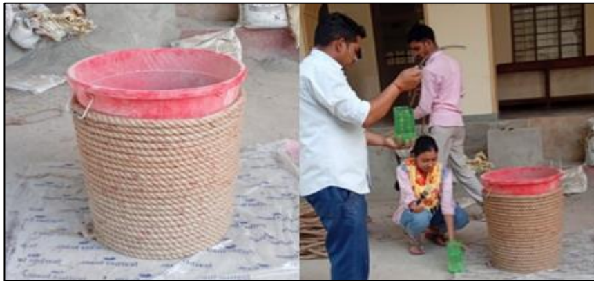
Figure 3-1 Dia of jute rope – 30mm and the size of the model – 1.5ft dia & 2ft height
