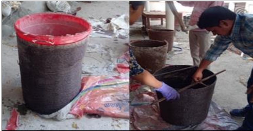
Figure 3-3 Dia of jute rope – 10mm and the size of the model – 1.5ft dia & 2ft height
