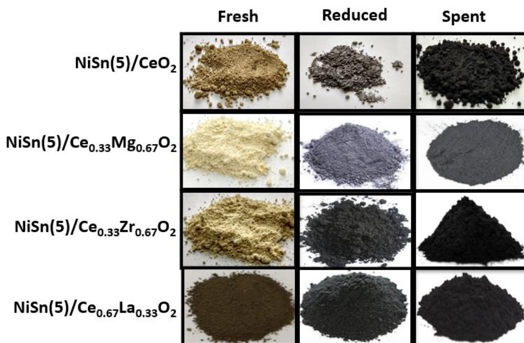
Figure 3. 12: Example physical appearance of NiSn(5)/CeO 2 , NiSn(5)/Ce 0.33 Mg 0.67 O 2 , NiSn(5)/Ce 0.33 Zr 0.67 O 2 , NiSn(5)/Ce 0.67 La 0.33 O 2 catalysts after preparation (fresh), reduction, and spent.
