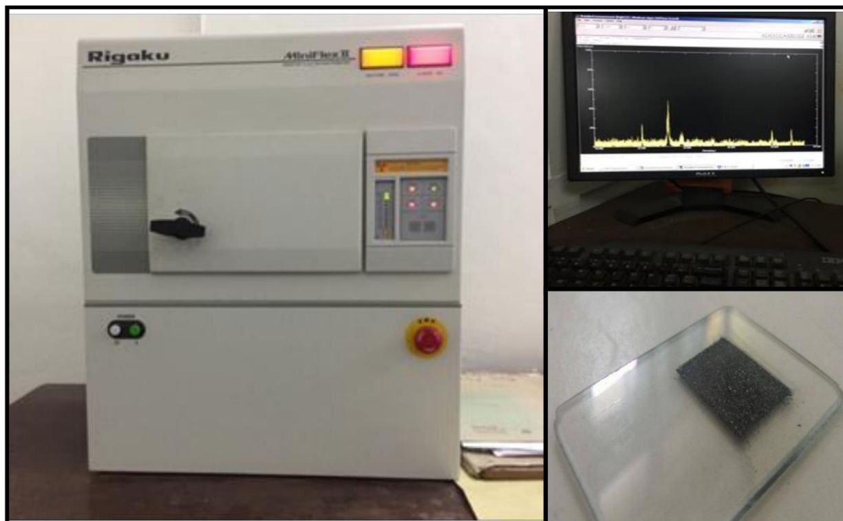
Figure 3. 13: XRD equipment used in for catalyst characterization along with the catalyst placed over glass sample holder.
