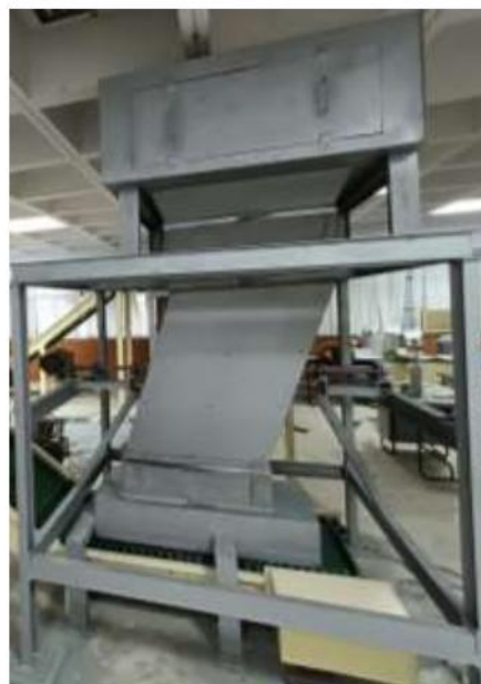
Fig. 6.14 Installation of transfer chute
