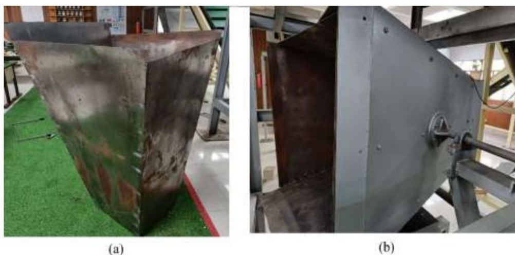
Fig. 7.7 (a) Fabricated conventional transfer chute (b) Conventional transfer chute inserted in the newly designed flexible chute
