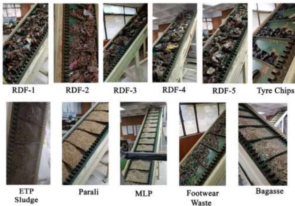
Fig. 7.2 Experiments for AFs received from the industry at varying mass flow rates
