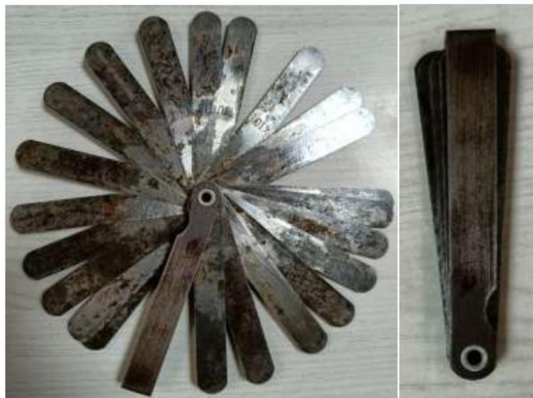
Fig. 6.25 26 blades feeler gauge used for measuring wear rate
