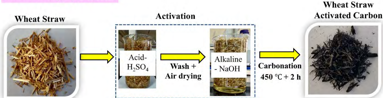
Fig. 4.2 Adsorbent preparation using physio-chemical treatment
