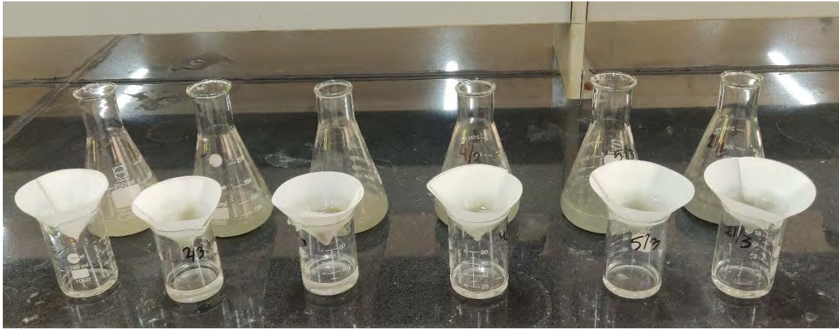
Fig. 6.8 Experiments performed for heavy metals leaching from mortar mixes
