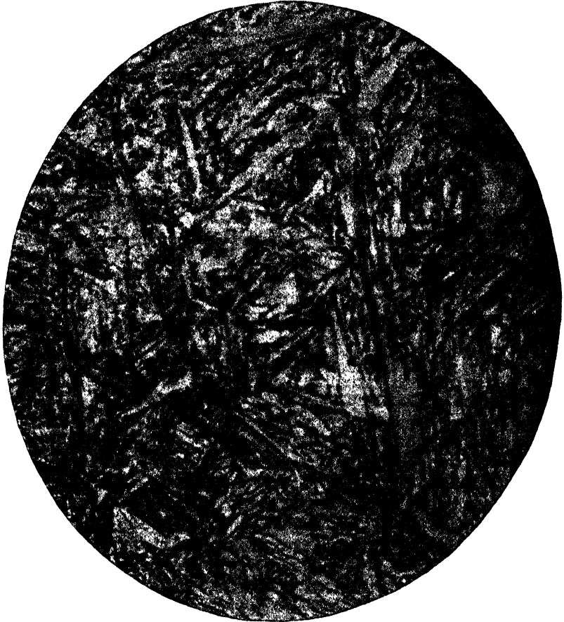
FIG. 15E. Martensite = the Hard Structure Produced When Austenite is Cooled at What is Called "the Critical Cooling Rate." 2000 \times . (Contrast this with Fig. 15C = the structure which results when austenite is cooled very slowly. The steel in this micrograph and that illustrated in Fig. 15C both contain 0.83 per cent of carbon.) (Courtesy Joseph R. Villela)
